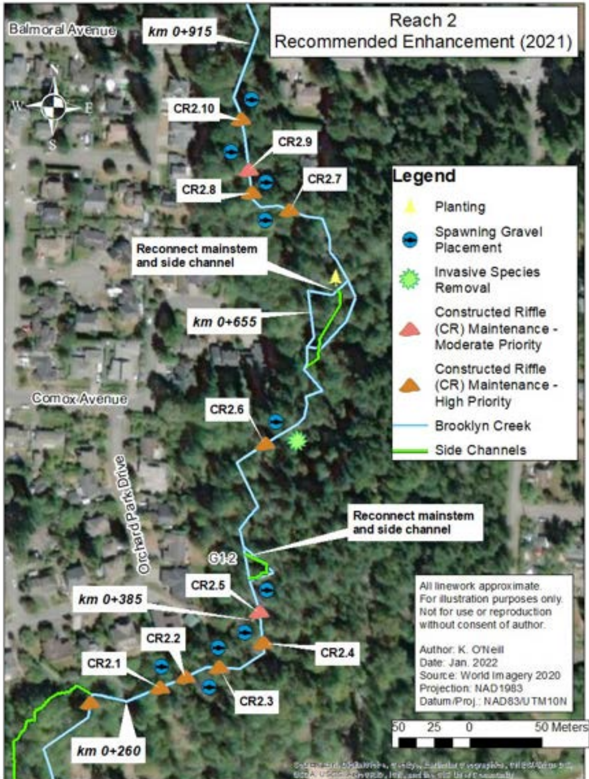
Figure 15. Reach 2 overview showing general locations of recommended enhancement projects. Invasive species removal should be conducted throughout reach (especially in areas where other enhancement/maintenance work is conducted) – invasive species removal symbol symbolizes entire reach.
