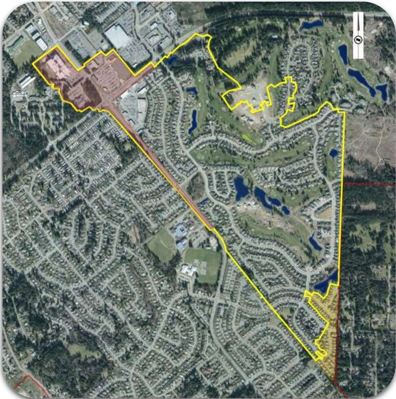
Figure 1 – Detention Pond 20 Catchment Area
